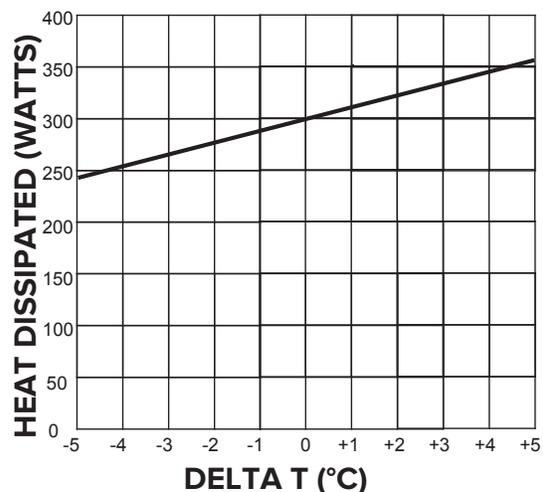
Note: Delta T is the temperature difference between the inside enclosure temperature to the outside enclosure temperature
