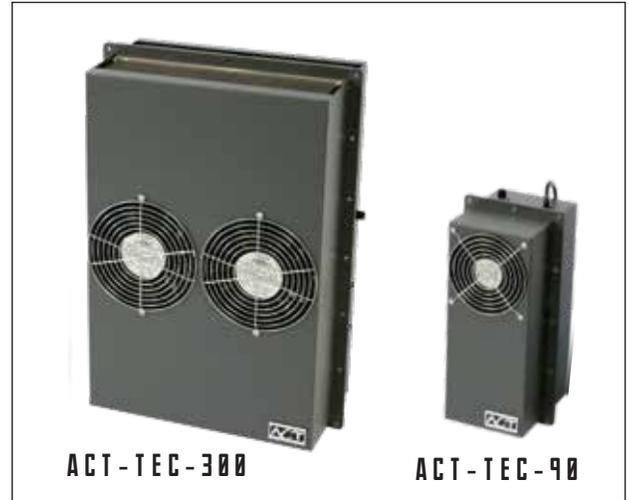
The ACT-TEC Thermoelectric Cooler series are compact solid state air conditioners. They cool the internal enclosure space with highly reliable Peltier cooling. The Peltier cooling cycle involves no moving parts, compressors, CFC refrigerants or circulating liquid. They feature a very long life as they are not vulnerable to refrigeration leaks. They exceeded the rugged industrial requirements of operating two four hours per day, seven days per week. In addition,
